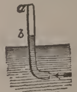
Pitot's Tube. a, bent glass tube; b, the level of water.
